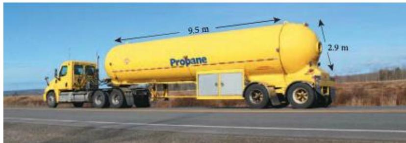
The tank on this truck consists of two hemispheres and a cylinder. The diameter is 2.9 m and the length of the cylinder is 9.5 m. Calculate the volume of the tank in megalitres.
