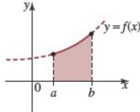
The solid generated is shown below and is symmetrical about the x-axis and any vertical cross-section is circular, with a radius equal to the value of  $y$  at that point. For example, the radius at  $x = a$  is  $f(a)$ .
