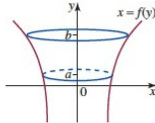
The volume of the solid of revolution is  $V = \pi \int_a^b [f(y)]^2 dy$ .
