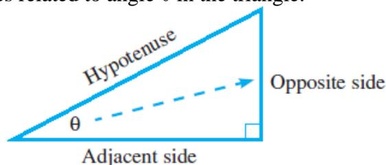
In trigonometry, three ratios are used: **sine**, **cosine**, and **tangent**. We will first investigate the **tangent** ratio, abbreviated to **tan  $\theta$** .
